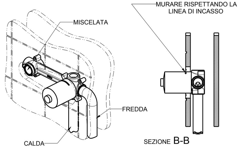
3) AVVITARE IL RACCORDO AL CORPO CON L' AUSILIO DI TEFLON PER GARANTIRE LA TENUTA
